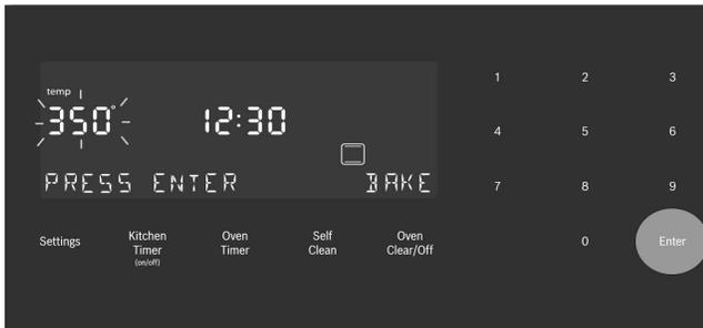
2. Press **Enter** to start the mode using the default temperature.
