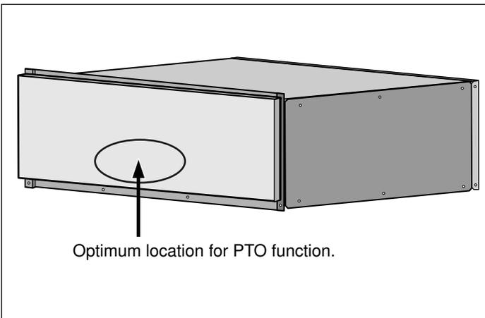
**Note:** It should be noted the recommended and optimum location for opening the drawer is the lower center front. The drawer will operate with an opening force applied to any location on the drawer front, however a slight increase in opening force may be required.
