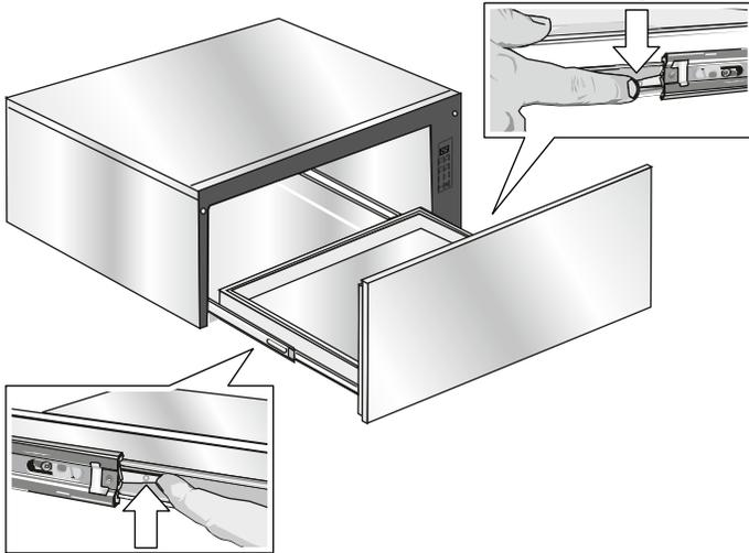
2. Grasp both sides of the drawer and pulling straight and level, carefully remove the drawer housing. This step may require light to moderate force to completely remove drawer.
