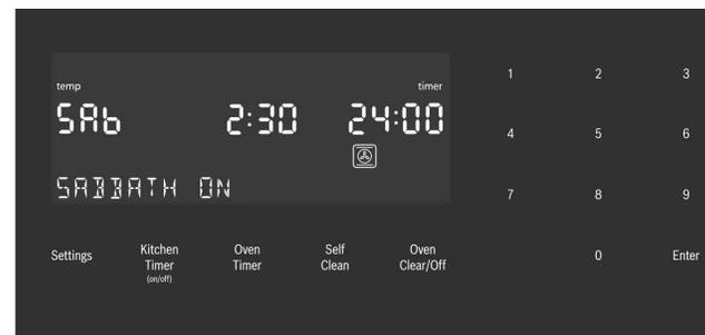
4. After the Sabbath mode countdown reaches zero, the oven displays the current time and the message “SABBATH”. No changes can be made at this point. To end the Sabbath Mode and return to normal function, press the **Oven Clear/Off** touchpad.
