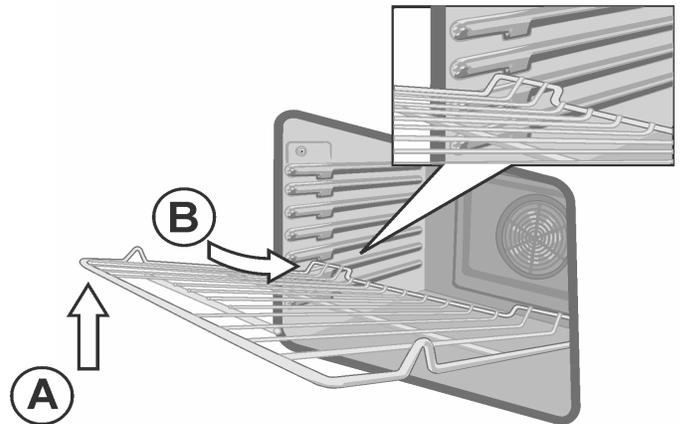
3. Tilt rack up (A) to allow the upwardly sloped rear of the rack to slide under the stop molded into the front portion of the rack guide above.
