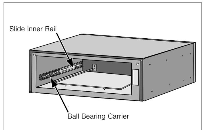
**Note:** The housing of your warming drawer should match the image below identically before starting your installation. The ball bearing carrier should be locked in to the inner rail's black plastic rail tip at the front of the inner rail.
