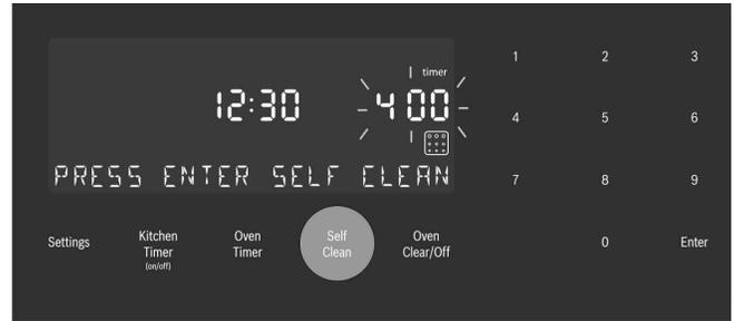
4. When the desired self-clean time is displayed, press **Enter** on the numeric keypad.
