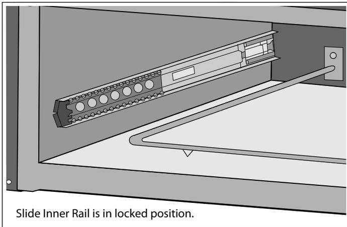
2. Position the drawer assembly in front of the housing assembly and align the rail (plastic rail tip) to the slide ball carrier assembly. Keeping the drawer assembly level and square to the housing, gently insert the drawer to the housing assembly.
