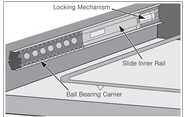
1. With the drawer removed, set the slide inner rail to the drawer locked position by pushing the slide inner rail **toward** the rear of the housing until it locks in place.
