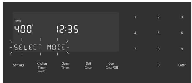
3. Press a Mode Selection Touchpad to select a cooking mode. The new mode and temperature set automatically after 10 seconds if **Enter** is not pressed.
