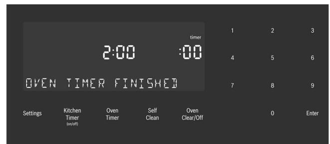
3. When the timer reaches :00 the cooking mode ends and the message "OVEN TIMER FINISHED" is displayed. The oven alarm tone sounds every 10 seconds for 2 minutes.
