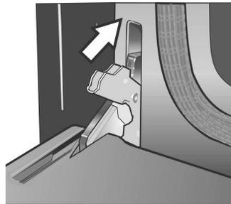
5. Push the levers on both the hinges up and forward until they are locked into the slot, flush with the front of the oven body.
