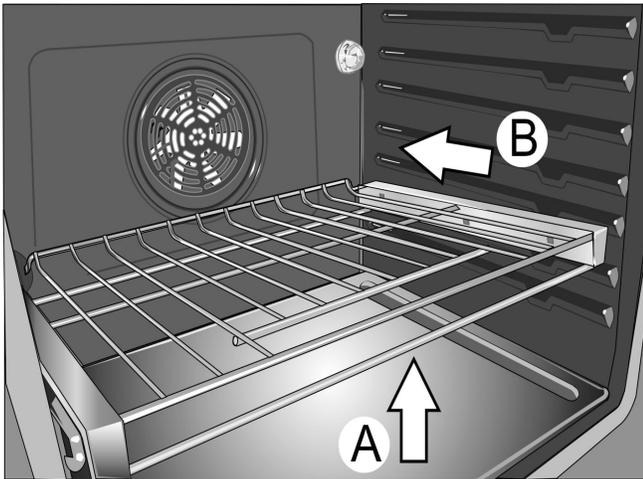
3. The back of the telescopic rack drops into place.
