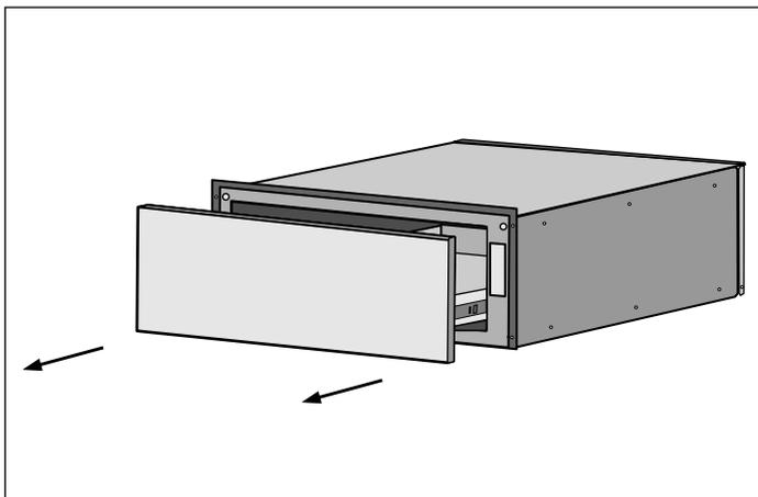
3. Install or service (clean) housing with drawer removed.
