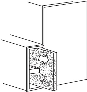
**Fig. 23 - Removal of Filter from Side Blower Cabinet**
